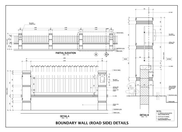
Fig 3.17: Sketch illustrating typical boundary fence treatments for industrial Plots
