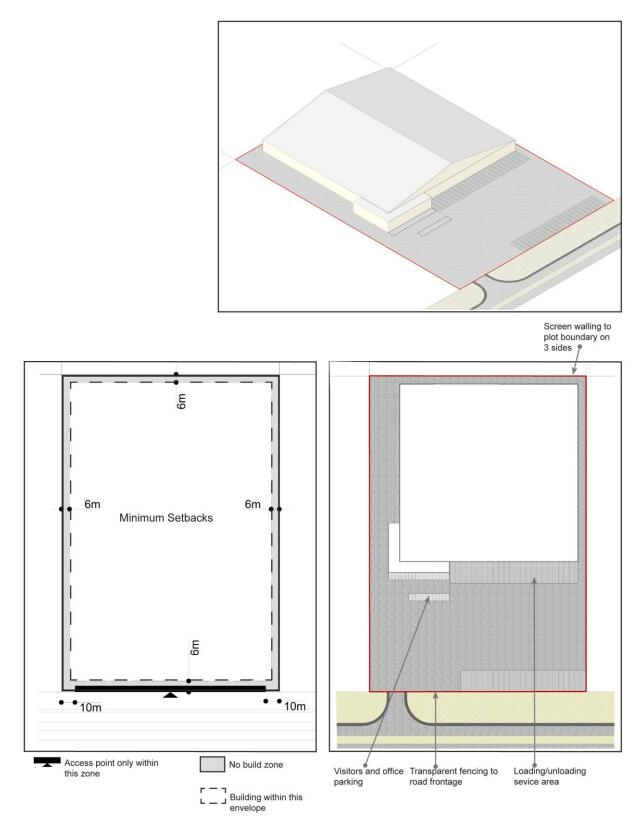
Fig.3.8: Setbacks, Access and Plot Coverage for General Industry -large warehousing units
