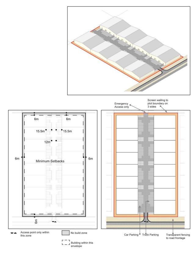
Fig.3.9: Access Arrangements around Junctions for General Industry -small warehousing units
