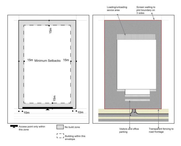
Fig.3.6: Setbacks, Access and Plot Coverage for Heavy Industry Plots)
